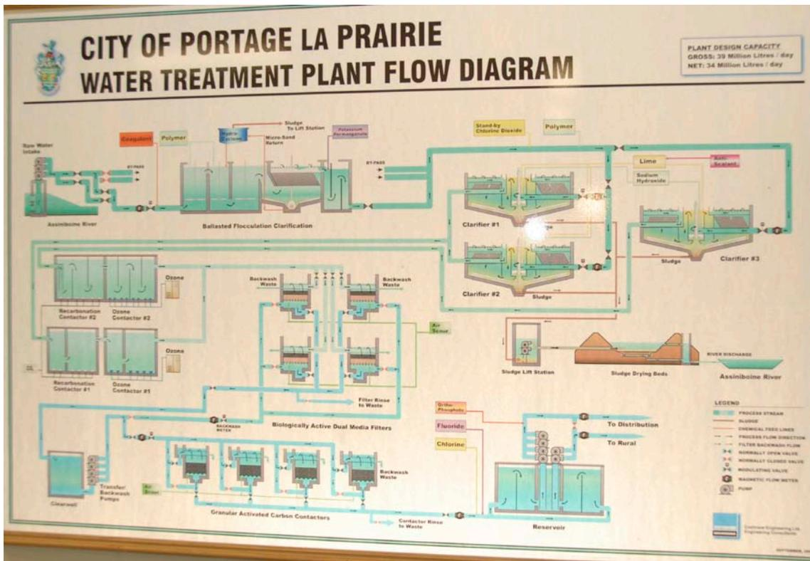
Figure A- 5 Water Treatment flow diagram
